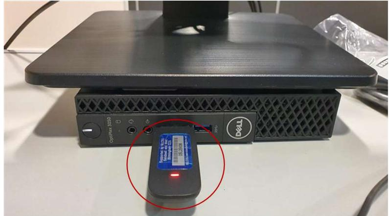
2. Unplug the 4G Dongle and wait for about 10-15 seconds and then plug it back in the USB port. You will see the light on the dongle turn from white to red.
